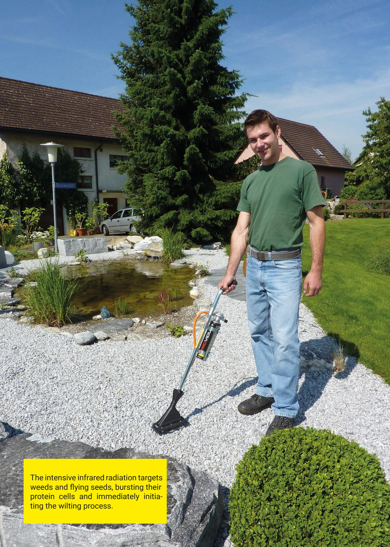
The intensive infrared radiation targets weeds and flying seeds, bursting their protein cells and immediately initiating the wilting process.
