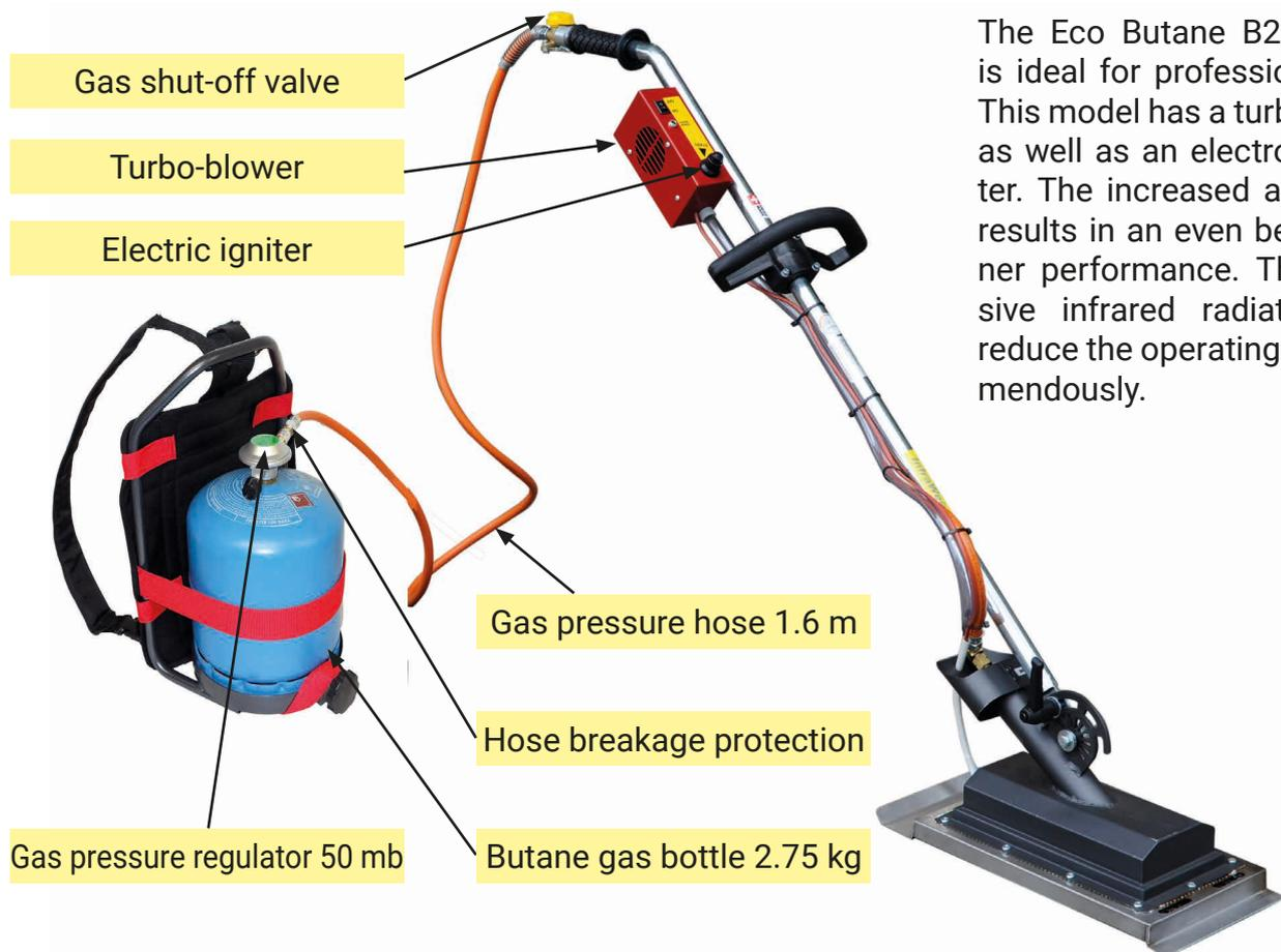
The Eco Butane B2R model is ideal for professional use. This model has a turboblower as well as an electronic igniter. The increased air supply results in an even better burner performance. The intensive infrared radiation can reduce the operating time tremendously.
