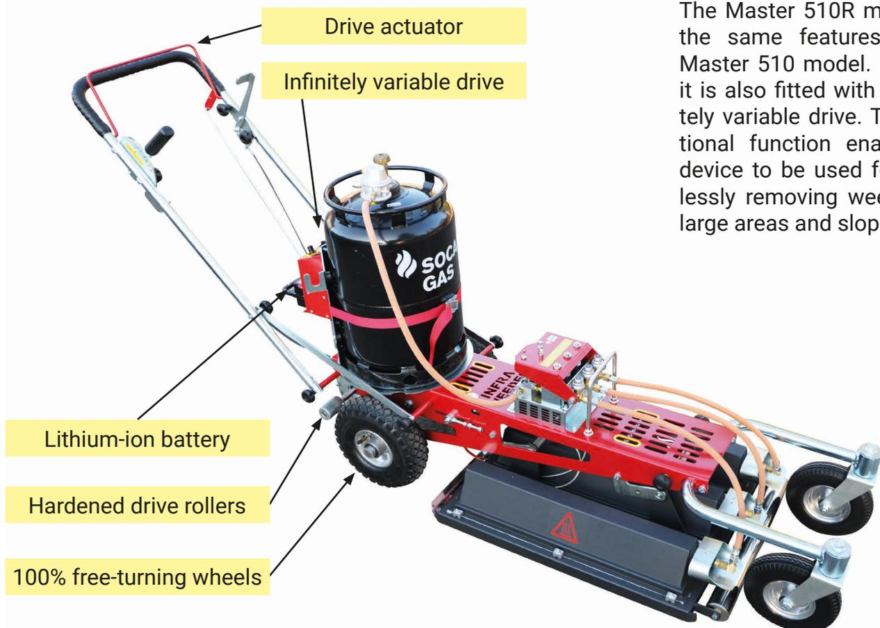
The Master 510R model has the same features as the Master 510 model. However, it is also fitted with an infinitely variable drive. This additional function enables the device to be used for effortlessly removing weeds from large areas and slopes.
